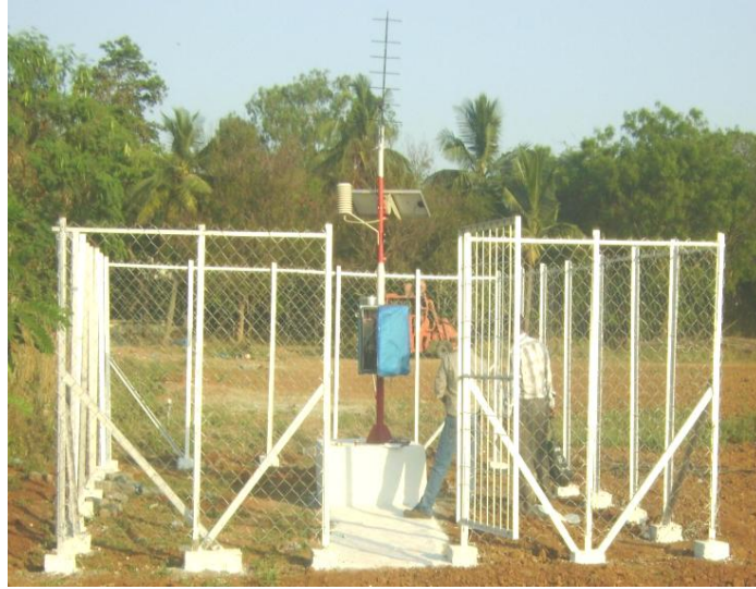
Fig.2 A typical ARG site at Krishi Vigyan Kendra, Kattupakkam
